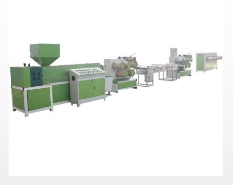
\*This step for producing PE or PP Flat yarn, one machine production per day can provide 3 netting machine material.
